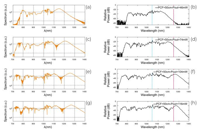
FIGURE 3. Supercontinuum spectra generated using 1.5 m of SC-3.7-975 nonlinear PCF. (a), (c), (e) and (g) Simulated results. (b), (d), (f) and (h) Experimental results for same fiber and coupled powers.
