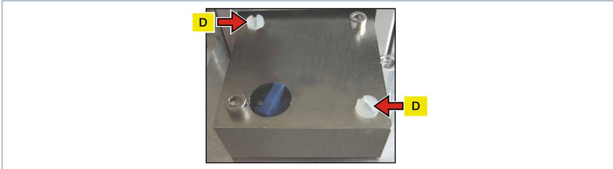
Fig. 16.3: Remove the plastic screws from the detector
