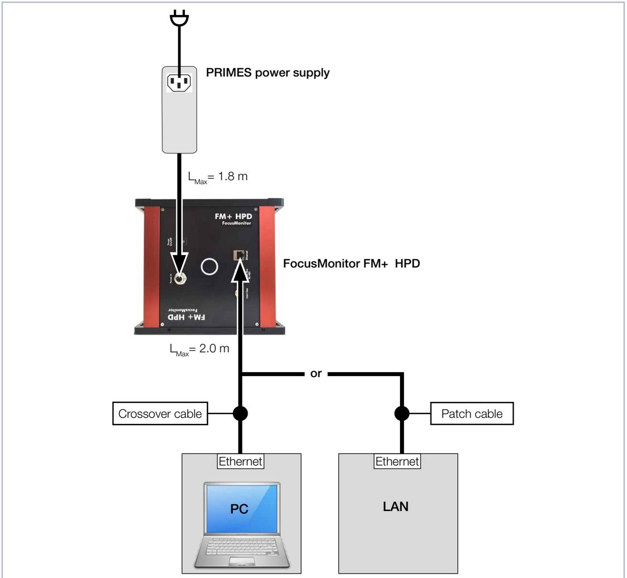
Fig. 9.2: Connection of FocusMonitor FM+ HPD
