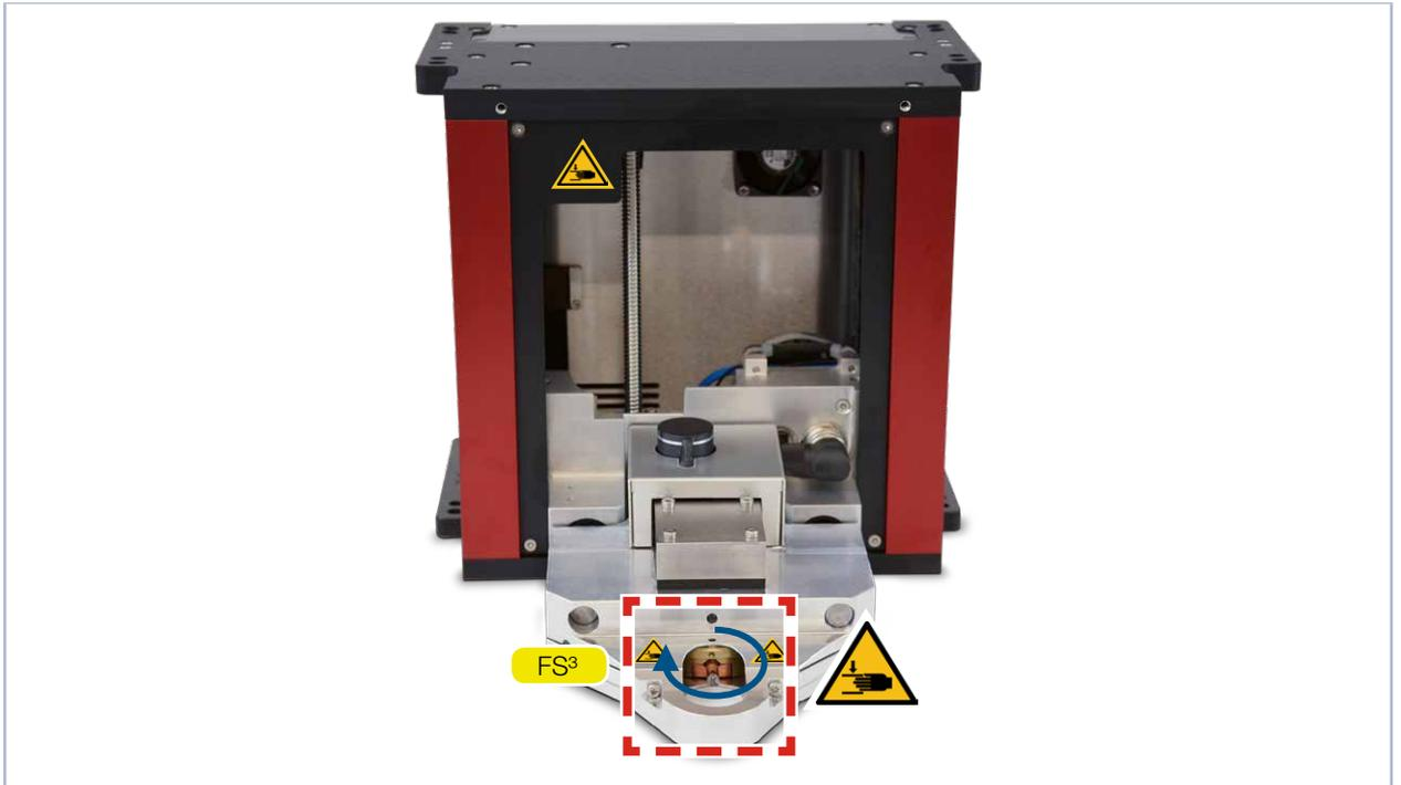
Fig. 8.1: Danger posed by rotating parts
