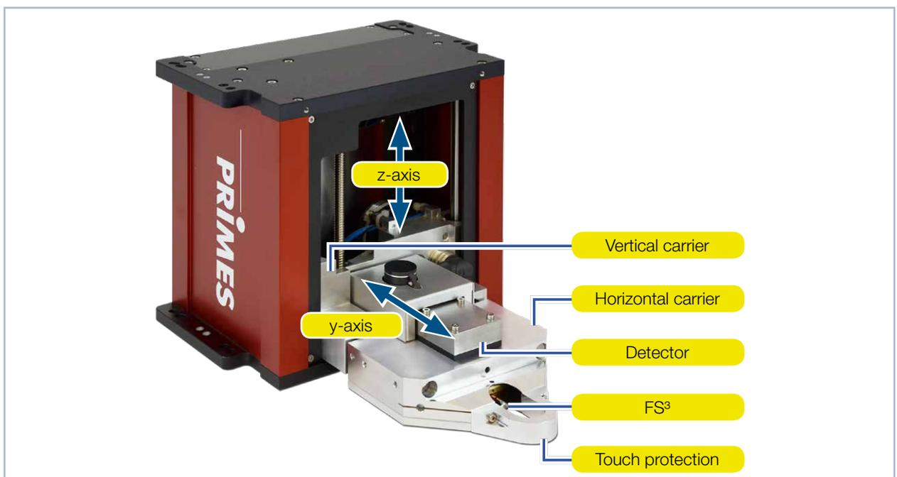
Fig. 5.1: Components of the FocusMonitor FM+ HPD
