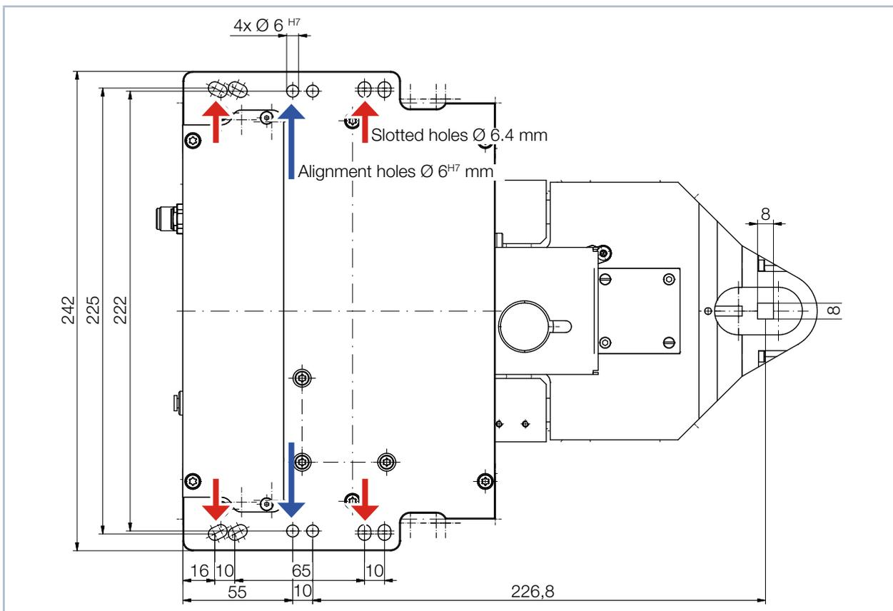
Fig. 8.9: Mounting holes, view from above (same hole pattern below)
