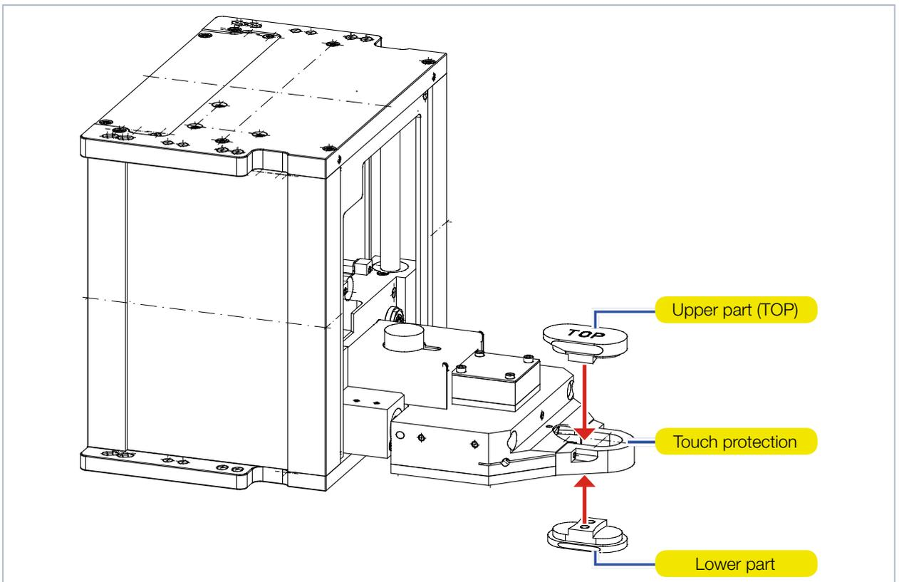
Fig. 8.5: Remove/insert the dust protection
