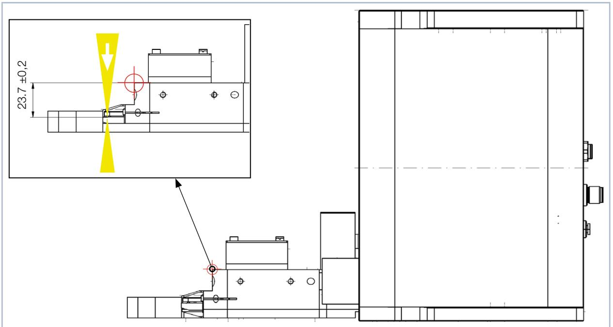
Fig. 12.1: Distance of the diffuser in the FS<sup>3</sup> to the horizontal carrier
