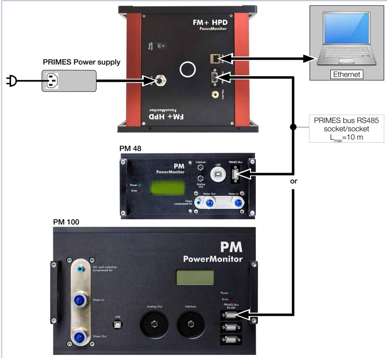
Fig. 9.3: Connection of the FocusMonitor FM+ HPD and PowerMonitor PM 48/100 to the PC
