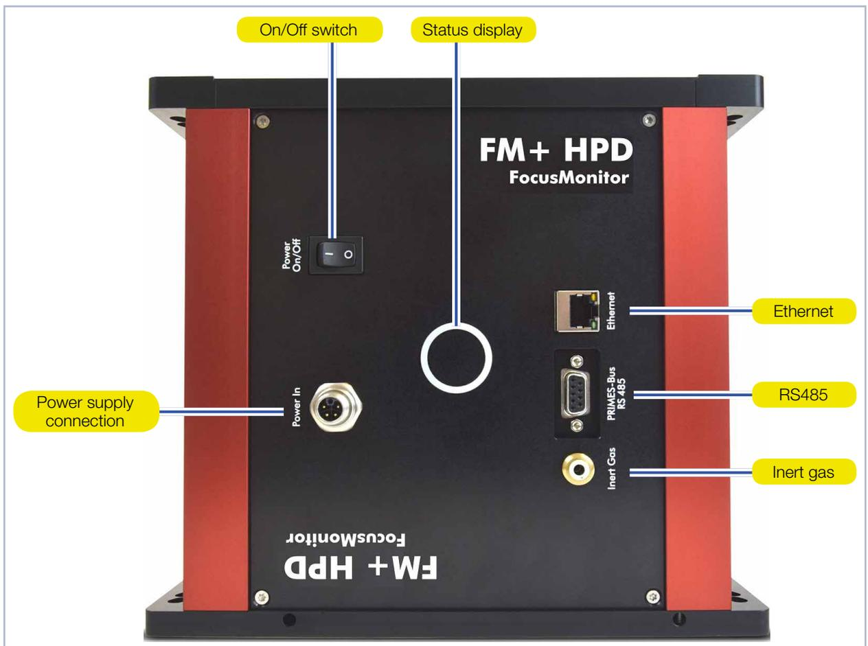
Fig. 9.1: FocusMonitor FM+ HPD connections
