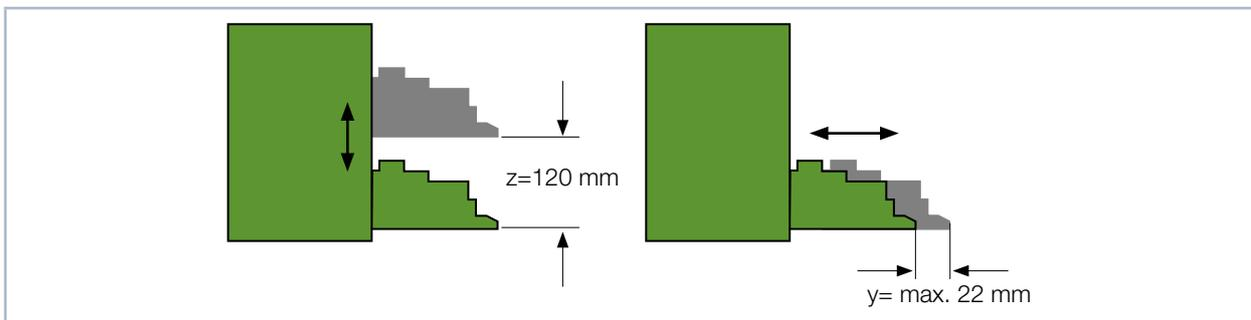
Fig. 8.3: Movement range of the horizontal and vertical carrier
