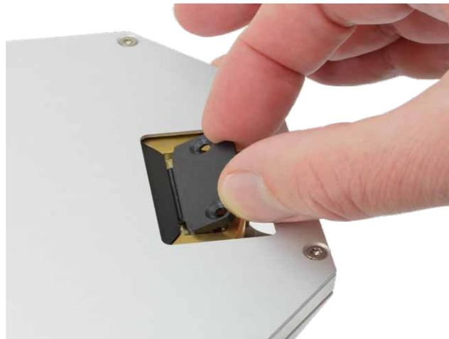
3. Insert the fastening screws (Torx T8) and tighten hand-tight.
