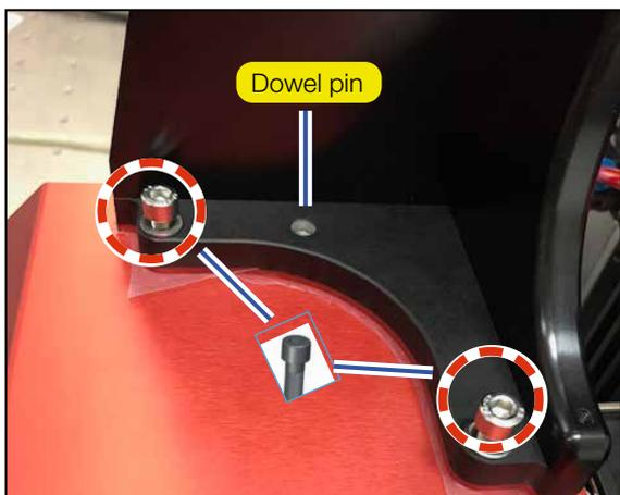
7. Fasten the fiber bridge by means of two screws (M5 x 10 mm) on both sides. Please note that longer screws (>10 mm) can block the Z-axis underneath.
