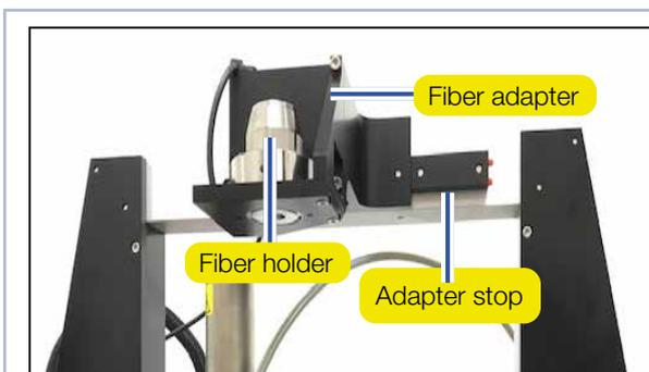
3. The position of the fiber adapter is fixed with the adapter stop. Press the fiber adapter against the adapter stop and tighten the screws.
