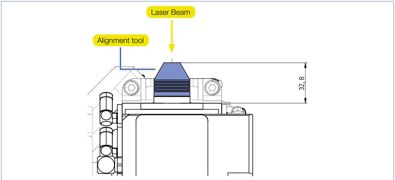
Fig. 7.4: Alignment tool for MSM+ HB
