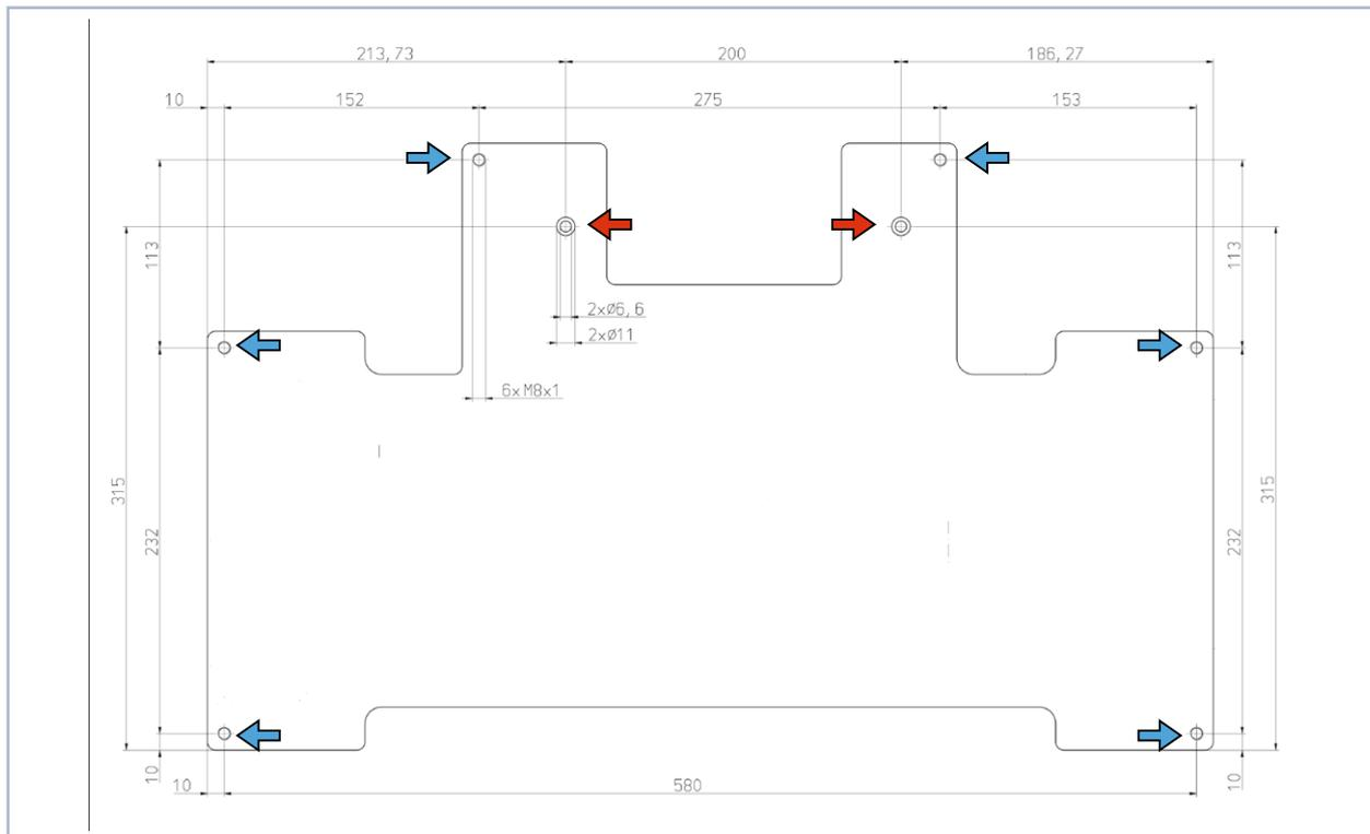
Fig. 7.6: Fastening bores MSM+ HB, view from above
