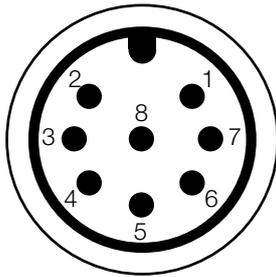
Tab. 8.2: Pin assignment of the safety interlock connector
