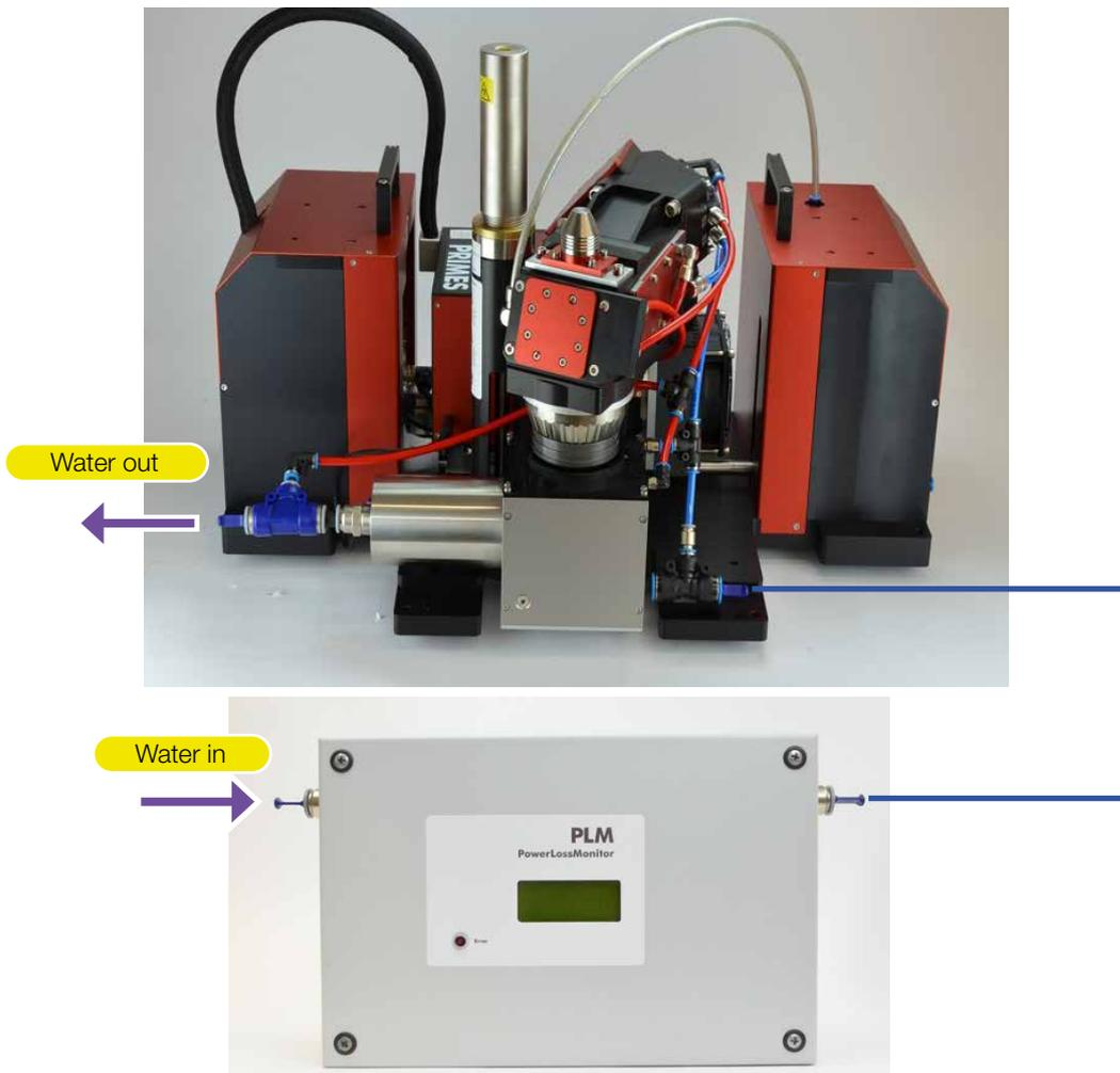
Fig. 16.1: Water connection (Figure shows PLM with MSM+ HB10)
