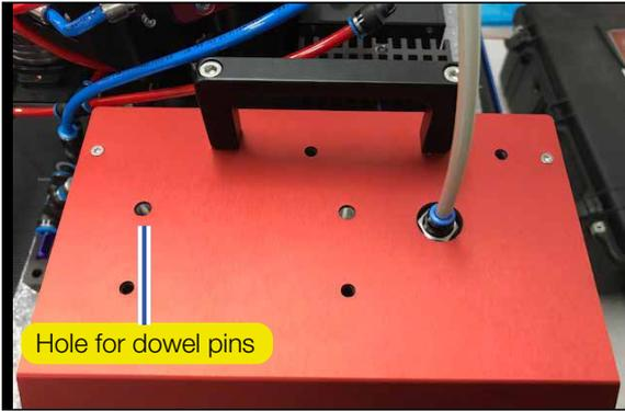
4. Insert the enclosed dowel pins on both sides into the hole provided.
