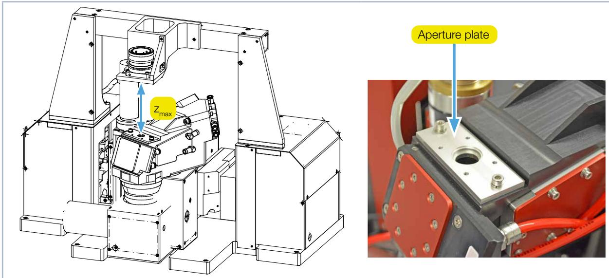
Fig. 9.1: Traverse range of the MSM+ HB with fiber bridge
