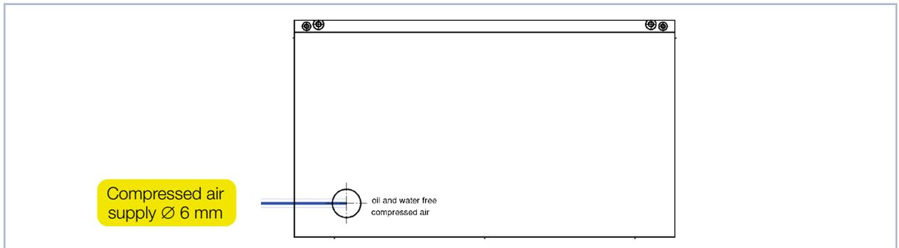
Fig. 8.6: Compressed air supply
