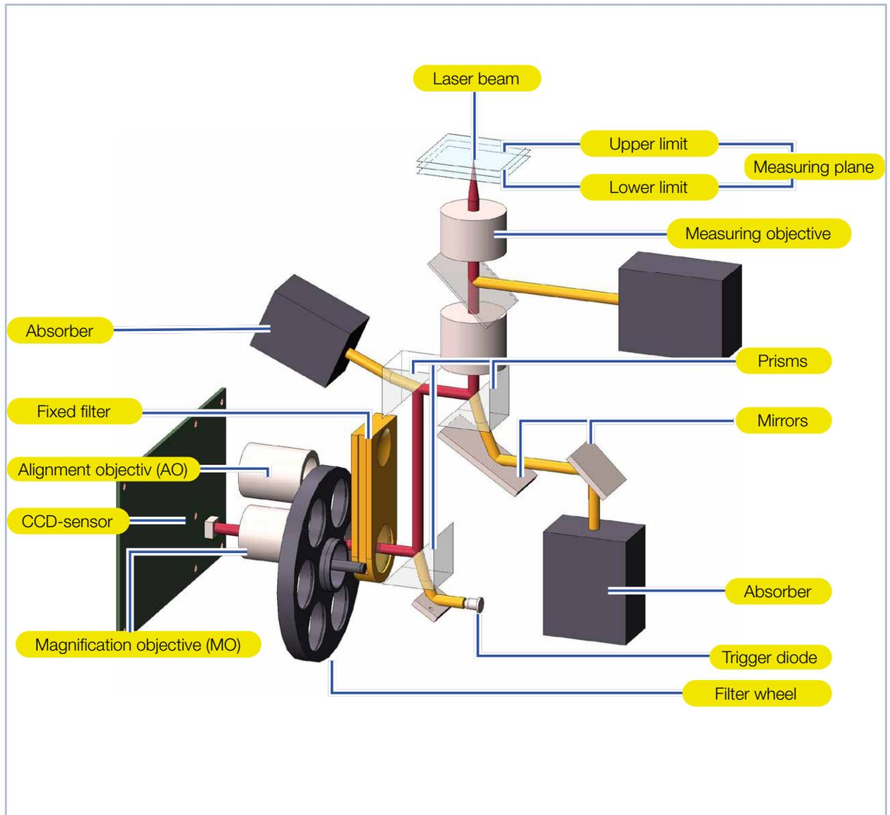
Fig. 4.5: Schematic illustration of the optomechanical design
