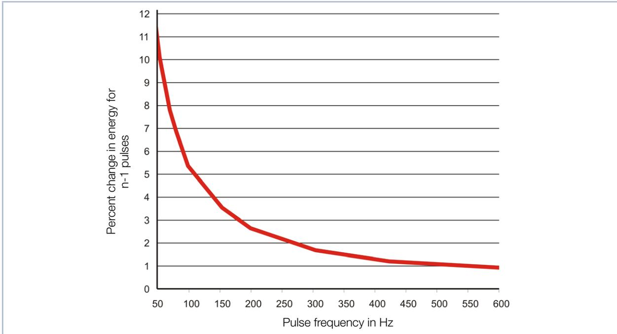
Fig. 16.3: Percentage of change in the detected energy when exactly one pulse is left out, in correlation with the pulse frequency
