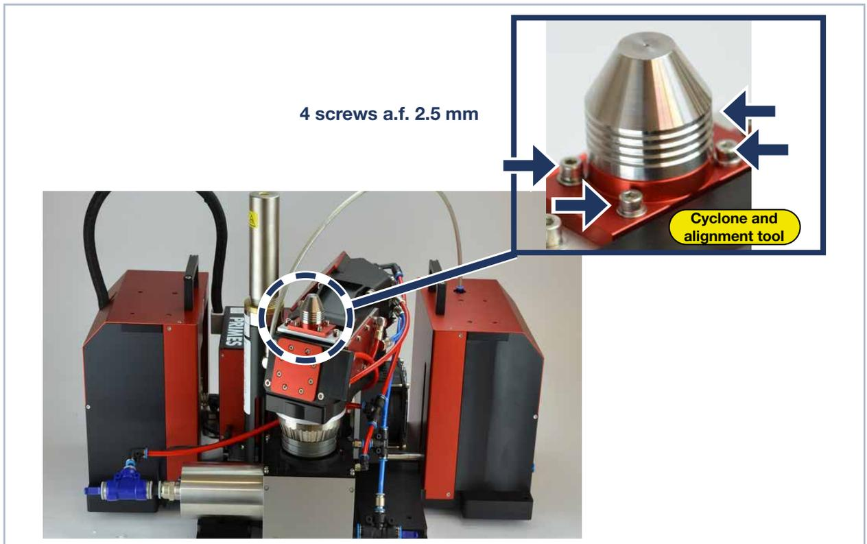
Fig. 7.2: Position of cyclone and alignment tool
