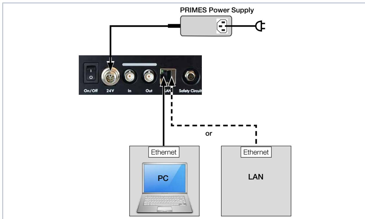
Fig. 8.3: Connection via Ethernet with a PC or a local network
