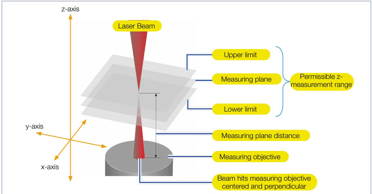
Fig. 7.1: z-measurement range of the MSM+ HB
