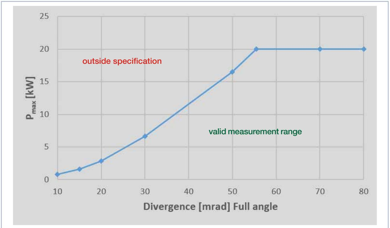
Fig. 4.6: Maximum power as a function of the laser divergence angle
