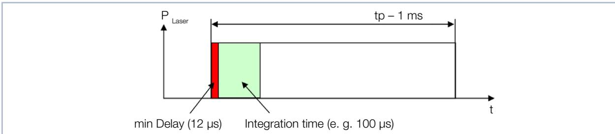
Fig. 16.6: Measuring parameters for pulsed laser systems with pulse duration greater than 1 ms
