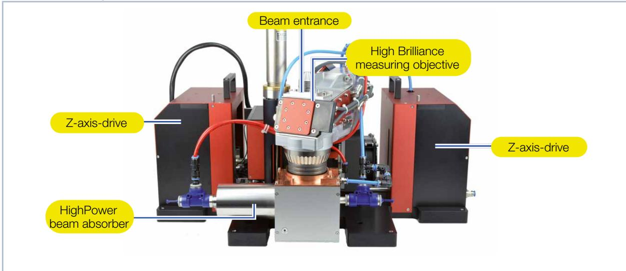
Fig. 4.3: Components of the MSM+ HB
