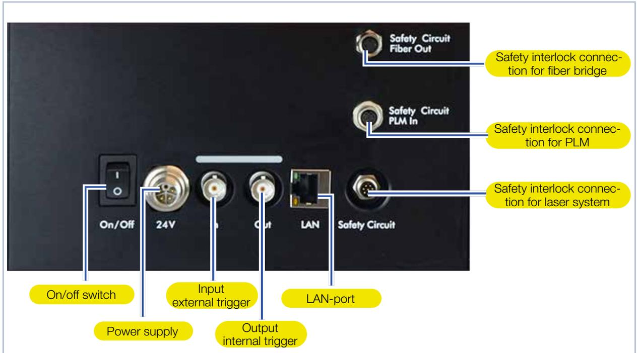
Fig. 8.1: Electrical connections at the device
