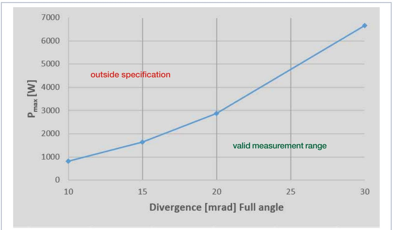
Fig. 4.7: Maximum power as a function of the laser divergence angle (excerpt)
