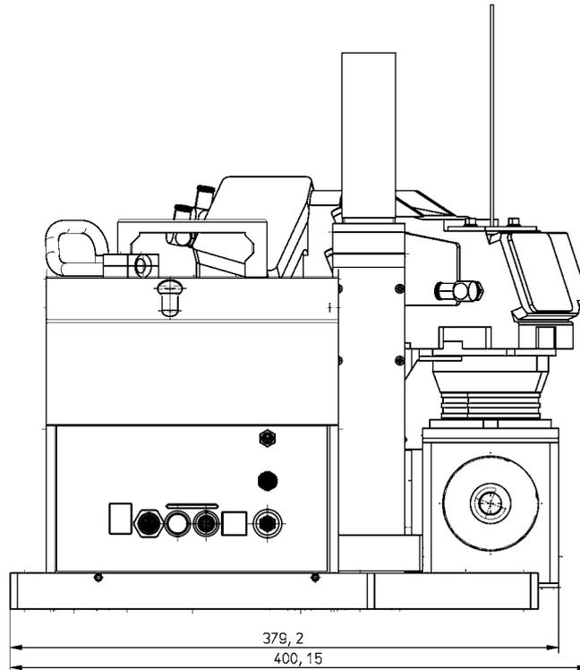
15.2 Dimensions of the MSM+ HB10 with fibre bridge
