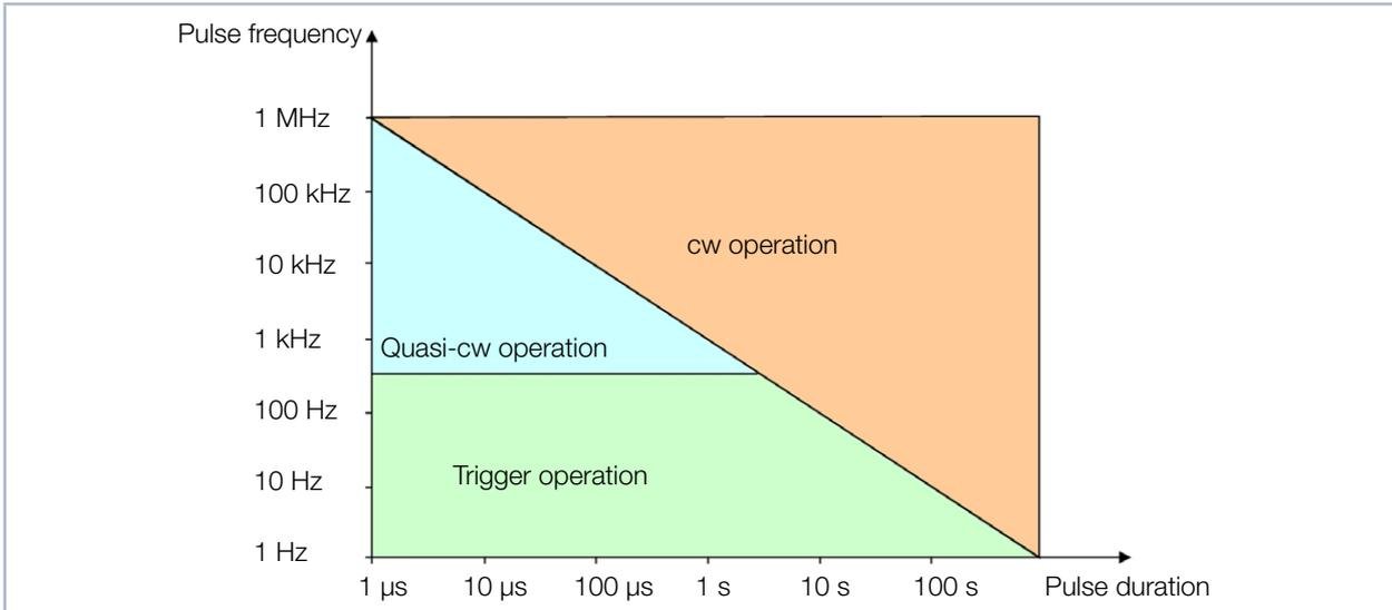
Fig. 16.5: Selection of the appropriate measurement mode based on laser parameters
