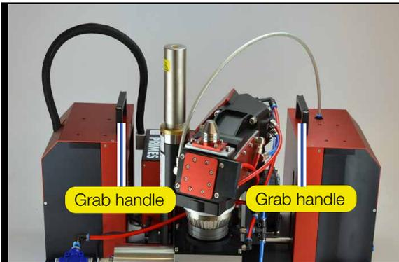
5. Disassemble the two grab handles on the MSM+ HB. To do this, loosen the visible screws in the grab handle.
