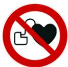
A possible hazard area for persons with pacemakers or implanted defibrillators is marked with a symbol on the device.
