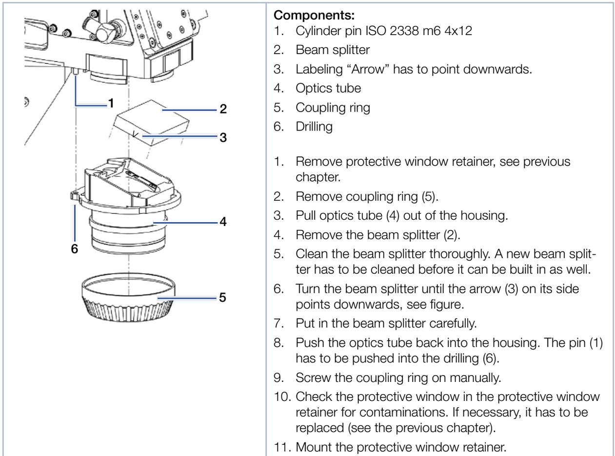
Fig. 11.4: Exchanging beam splitter
