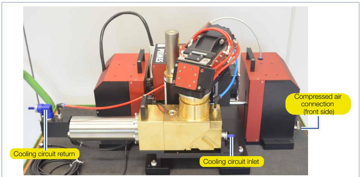
Fig. 8.2: Water and compressed air connections at the MSM+ HB20
