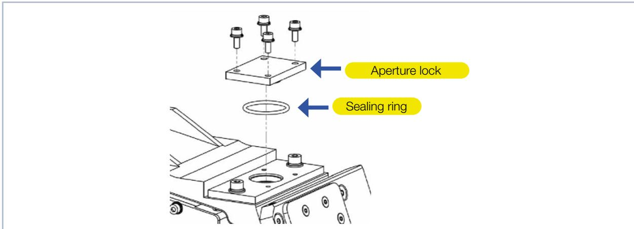
Fig. 7.3: Aperture lock at the beam entrance
