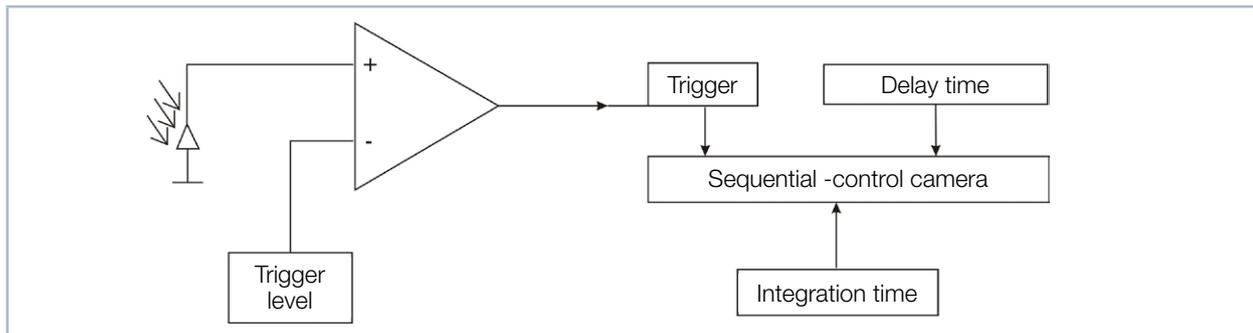
Fig. 16.2: Options for affecting the sequence control of the CCD sensor
