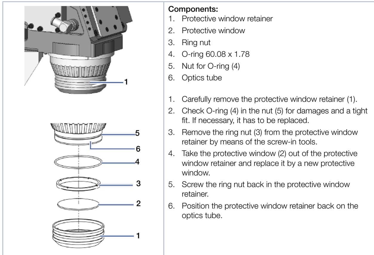
Fig. 11.3: Change of the protective glass in front of the power output opening (on a 10 kW unit)
