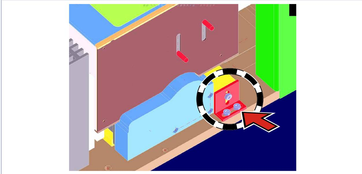
Fig. 6.1: Position of the transport lock at MSM+ HB10
