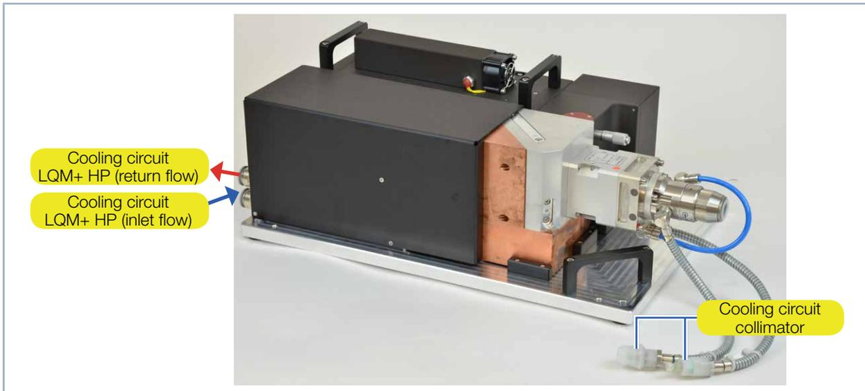
Fig. 19.1: Water connections
