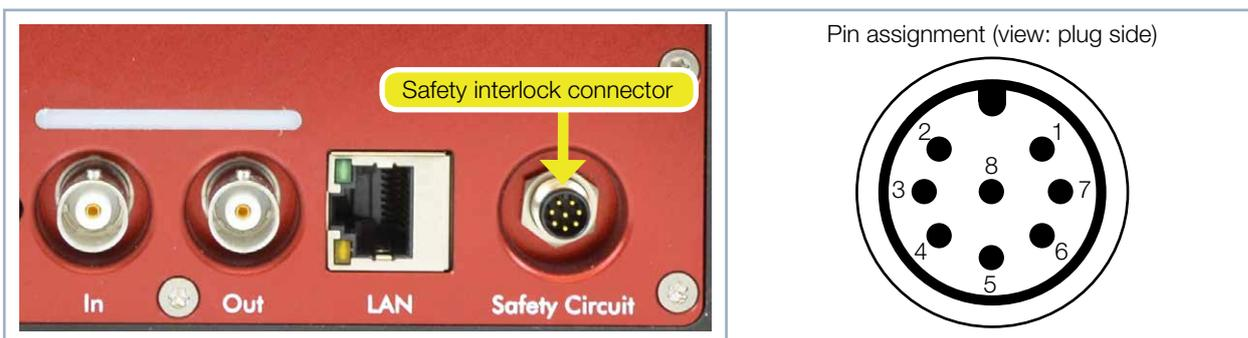
Fig. 9.5: Safety interlock device plug in the connection panel
