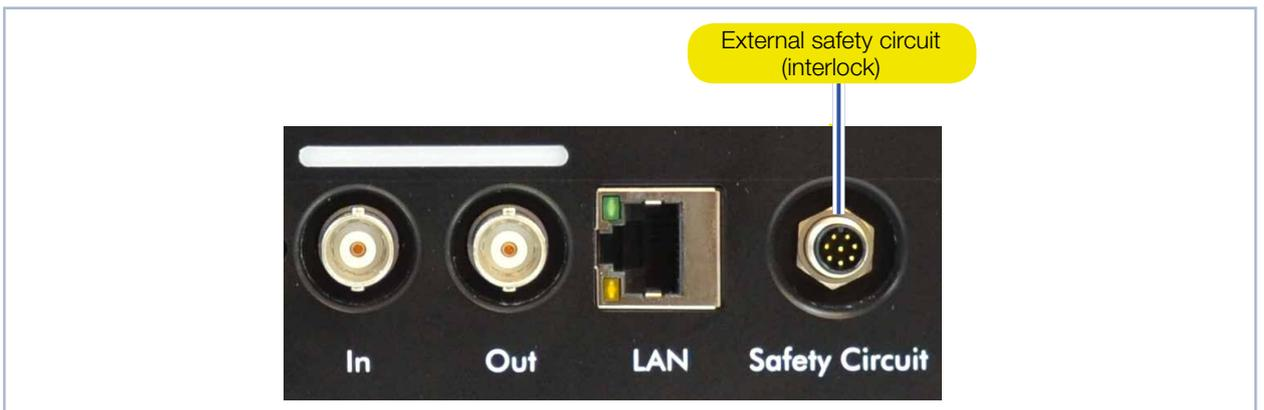
Fig. 10.5: Device connector of the external safety circuit
