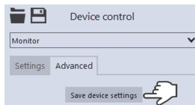
Tab. 12.5: Options in the **Device control** > **Advanced** tab of the **Monitor** measuring mode
