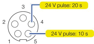
Pin diagram socket (top view, plug-in side)
