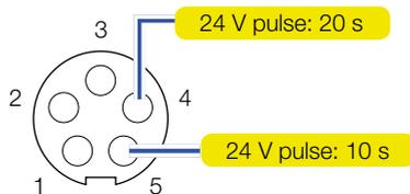
Pin diagram socket (top view, plug-in side)
