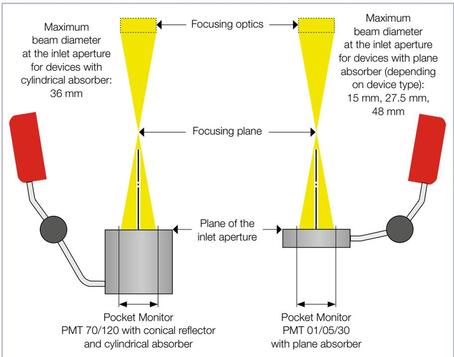
Fig. 9.1: Alignment to the laser beam
