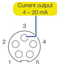
Pin diagram socket (top view, plug-in side)
